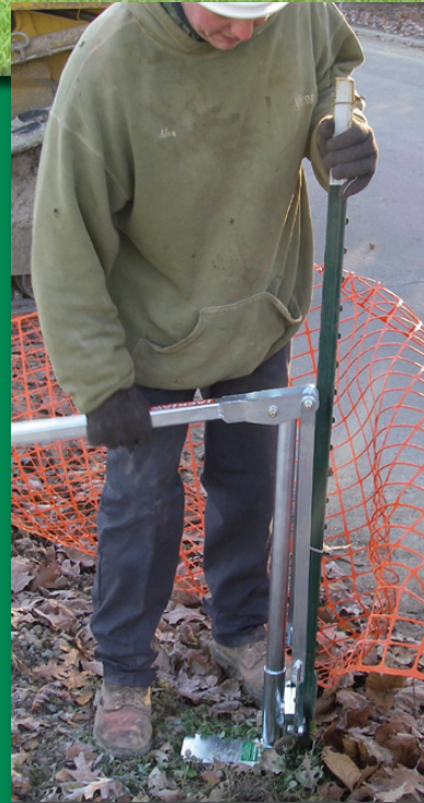
Pulls T-posts for construction, traffic and event barricades
